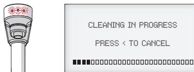
Flashing lights and progress bar shows cleaning is in progress
