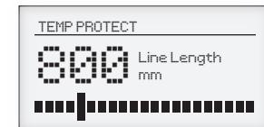
3. Use the adjustment dial to change the TEMP PROTECT value to match the measurement taken in STEP D of the Installation Procedure on page 13;
